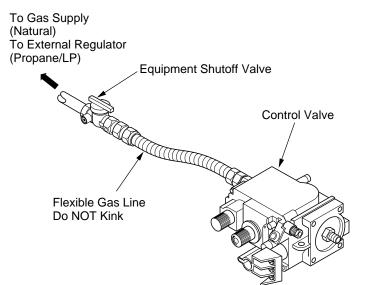
Figure 32 - Connecting Flexible Gas Line to Millivolt Valve
